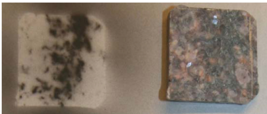
Figure 3: (left) Autoradiography analysis of core D7.1 from borehole KA3065A03 and (right) photograph of the same core. The core was drilled and sampled after the finalisation of the Long Term Sorption Diffusion Experiment (LTDE-SD) at Äspö (Sweden). The basis of the slice is approximately 16 mm. The blackening on the autoradiograph represents radioactivity of primarily cesium ( Cs-137 ). Figure reproduced with permission from Nilsson et al. [19].
